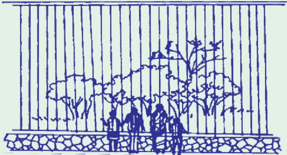
Piano string barrier
